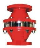
Flame arrester are safety device designed to extinguish or check the travel of flame in pipelines and ducts and to prevent flame spreading from them into or put of plant and equipments elements are stainless steel with a cast aluminium, carbon steel or stainless steel casing.
